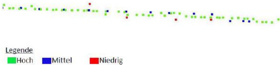
Figure 3-2: 10cm section through a section of road with different coloured point clouds depending on setting parameters for the evaluation
